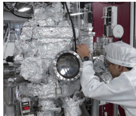
MBE装置を用いたCIGS太陽電池の作製 Fabrication of CIGS Solar Cells using Molecular Beam Epitaxy system
