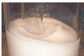
偏心二重円筒容器内の 非線形液面揺動 Nonlinear liquid oscillation in a cylindrical tank with an eccentric core barrel
