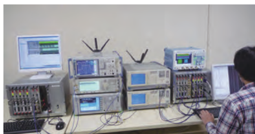
信号処理を駆使した無線信号伝送の実験系 Experimental System for Wireless Data Transmission Exploiting Signal Processing Techniques.
